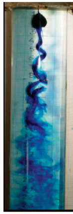
PL. (9 a) The wake instability for filling & emptying of the bubble. ( Re = 1787 , \Omega = 2.48 & L/R = 24 )
